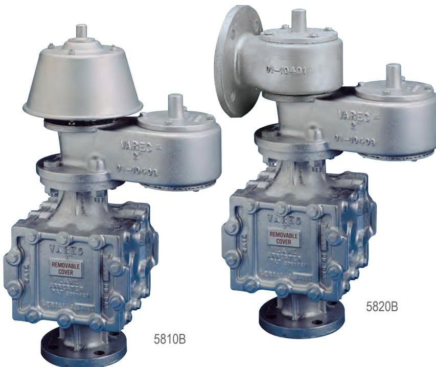
The flame arrester is designed to stop the propagation of a flame by absorbing and dissipating heat through the surface area of the bank sheets. Heat is absorbed as ignited gas attempts to pass through the small passages within the bank assembly. This action lowers the temperature of the gas below its ignition point and quenches the flame.
