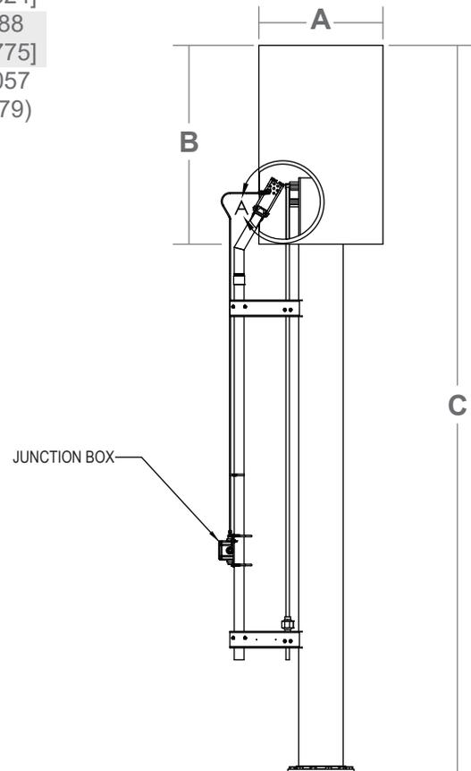
NOTE: Standard height of the flare stack is 15 feet to meet the minimum requirement per ANSI / CSA B149.6. The actual flare tip must be determined based on radiant heat at ground level. Consult factory for assistance. Stack dimensions are the same for all the options available with the 244WS or 244WL.
