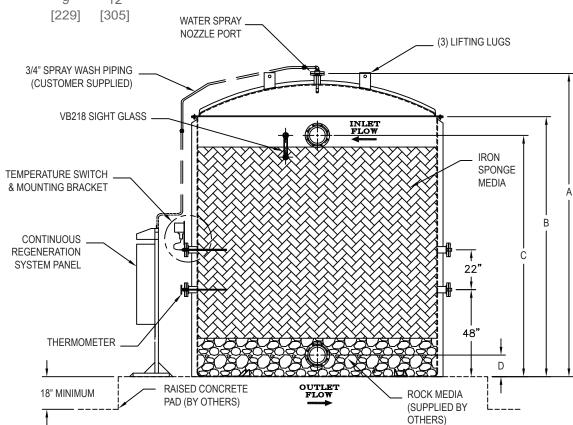
NOTE: Inlet and outlet pipe locations are subject to change, depending on the size of the pipe and flange.
